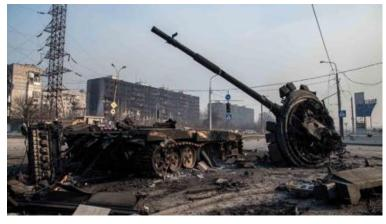
killing the crew. The "turret toss" occurred with roughly half of Russian tank losses and was not limited to the oldest tanks, as both the original unupgraded T-72 and newly upgraded T-72B3 Obr 2016 tanks suffered from similar rates of the "turret toss" occurring. The lack of improved survivability in newer upgrades of the T-72 demonstrates that the new version of Kontakt 5
